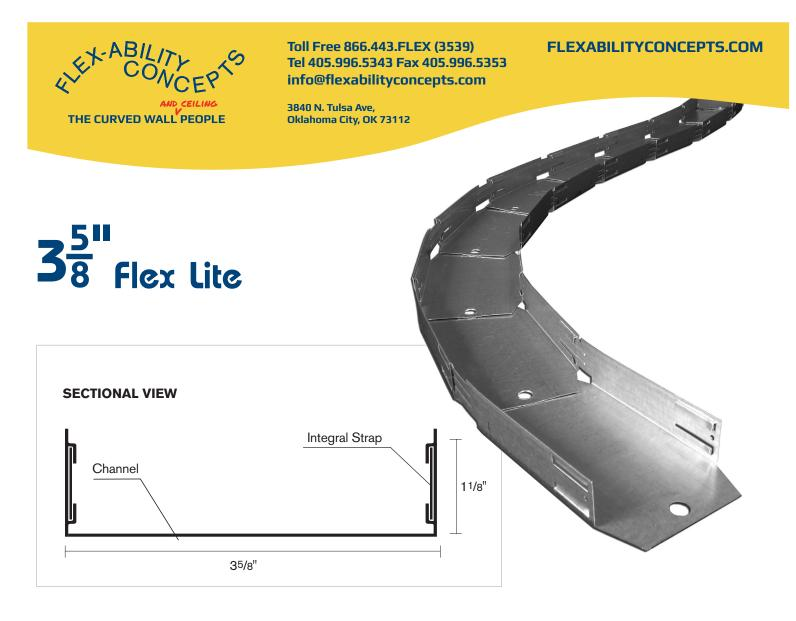
Flex Lite is the economical alternative to Flex-C Trac. Manufactured in an economical fashion, Flex Lite has been designed for curved framing applications where lateral loads are not an issue and where the higher quality of Flex-C Trac is not needed.
