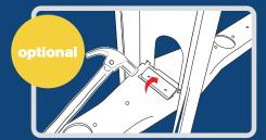
**For maximum speed and efficiency,** install Snap Lock as studs are being stood into place to achieve a 16" or 24" layout. **Next,** fasten the top and bottom of the studs.
